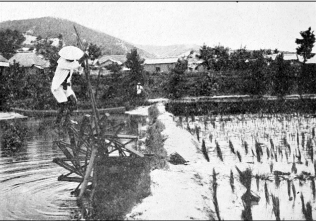
Fig 173 — Japanese irrigation foot wheel.
